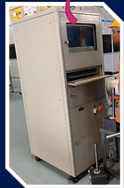
Eddy current Tester For Material Mix-up Identification
