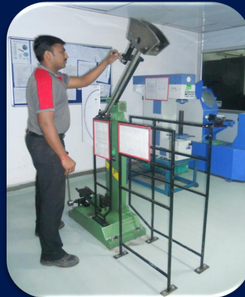
Impact Testing Machine - Up to -80°C
