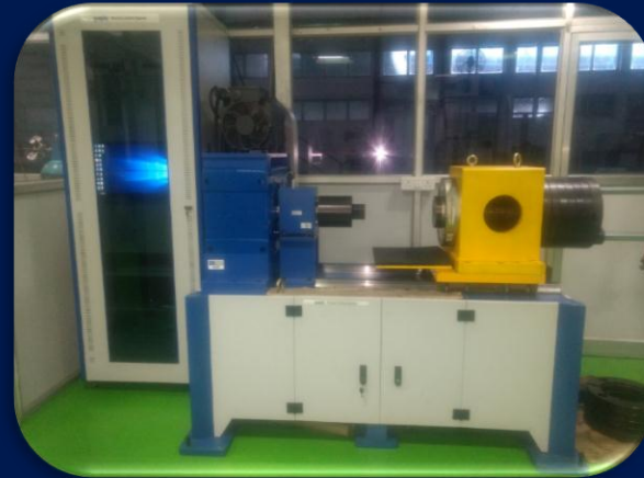
Torque Tension Testing Machine Capacity – up to M72
